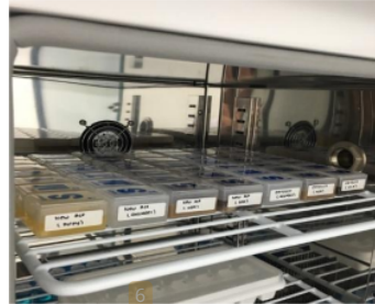
Figure 3. The sample was immersed in an incubator at a constant temperature of 37°C
