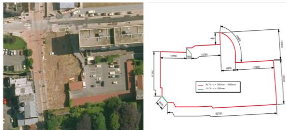
Figure 5. Plan of the construction site of the block of flats with an AZ 18 sheet pile wall that surrounded the excavation during the construction phase and was subsequently left in place to serve as the outer wall of the underground car park
