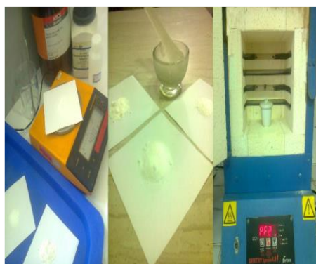
Figure 1. Different stages of synthesis by Eutectic method
