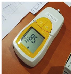
Figure 2 Portable analyzer operator ® Accutrend plus by Roche to Assess Lactic Acid
