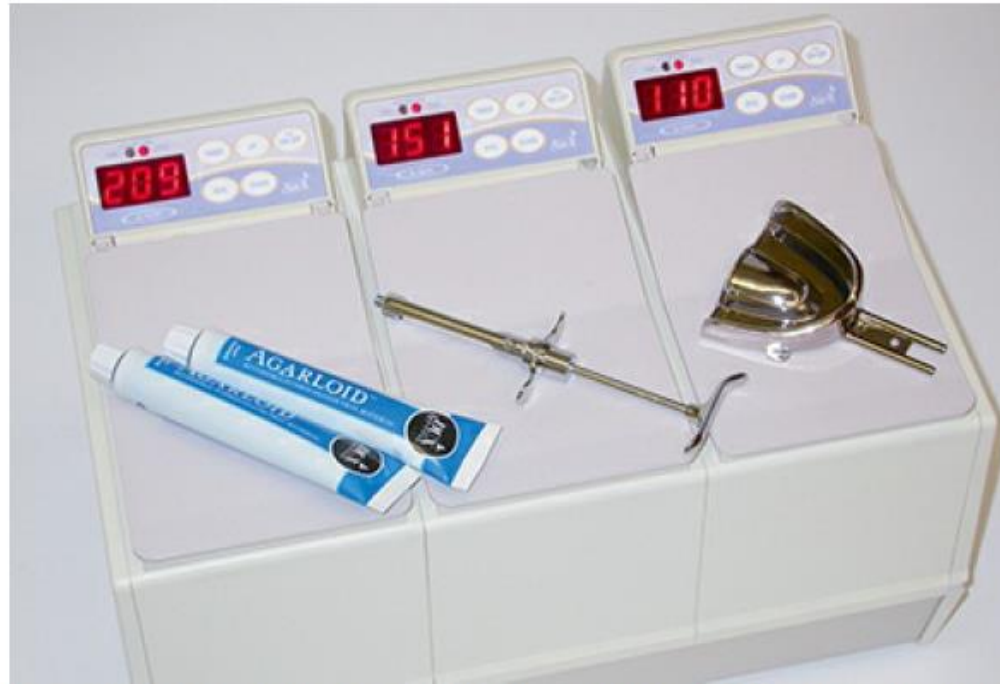
• FIGURE 13-13 Conditioning unit for agar impression materials. The three compartments are used for liquefying the material (left), storing after boiling (middle), and tempering the tray hydrocolloid (right). The number on the display shows the temperature setting in °F. Also shown in the figure are the tray hydrocolloid, a syringe for injecting hydrocolloids, and an impression tray. Note that the two tubes extending out from the handle of the tray are for water circulation.
