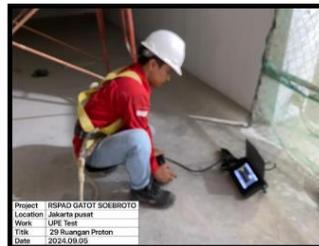
Gambar 29 Pengetesan *Ultrasonic Pulse Velocity* (UPV)
