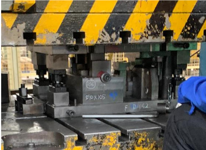
Gambar 4.12 Proses Pengetesan Dies Proyek D37 Exhaust Hanger
