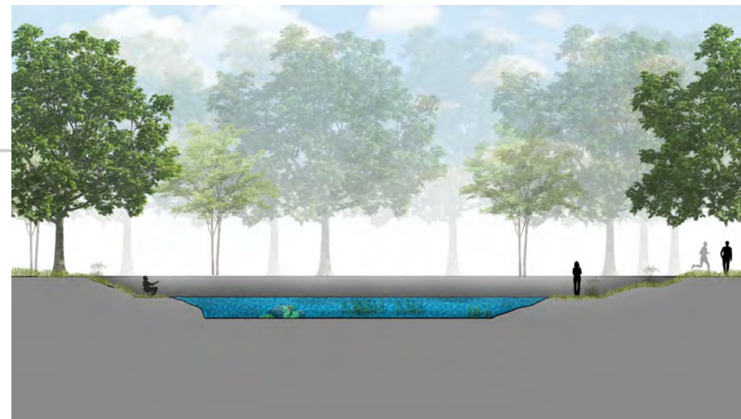
Bioswale Section Scheme
