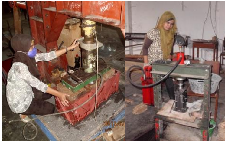
Gambar 4.20. Proses pengempaan beton polystyrene
