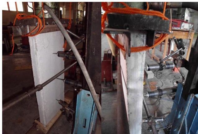
Gambar 4.29. Pengujian kuat tekan panel dinding polystyrene
