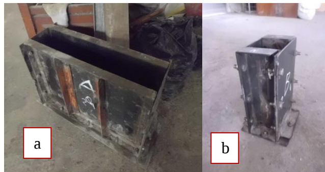
(a) Bekisting balok, (b) bekisting kubus
