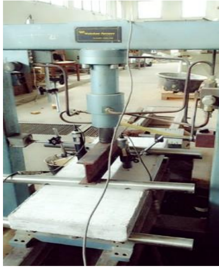
Gambar 4.27. Pengujian kuat lentur horizontal panel dinding polystyrene
