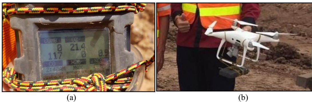
Figure 1. Tools for measurement a. Gases measured by MSA Altair 5x; b. Drone used to carry
