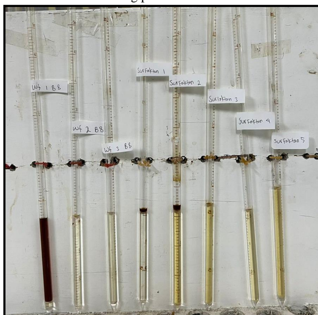
Figure 5. Oil recovery during ABS surfactant coreflood
