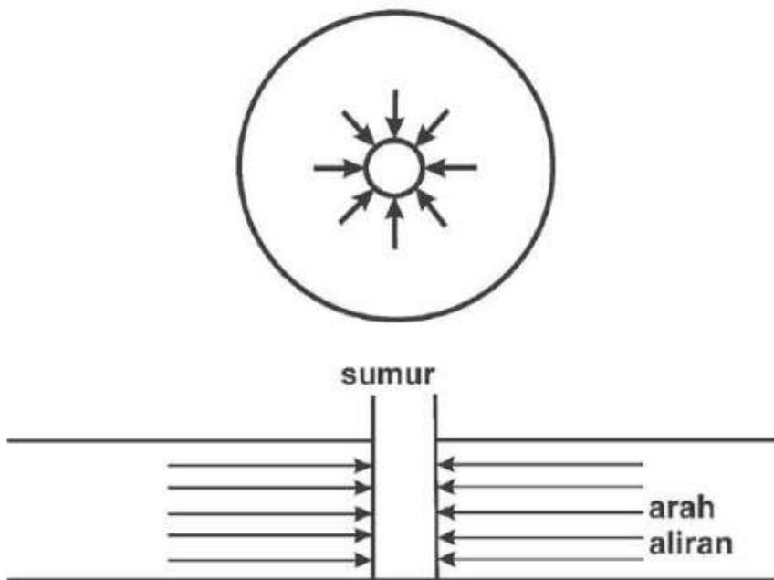
Gambar 5. 1 Aliran radial
