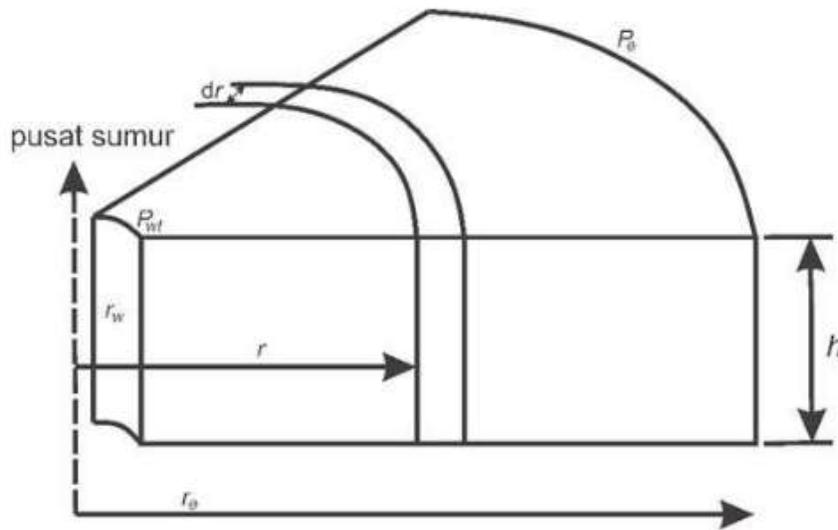
Gambar 6. 3 Aliran Radial
