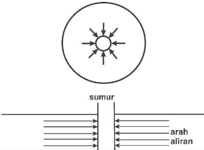
Gambar 5. 1 Aliran radial
