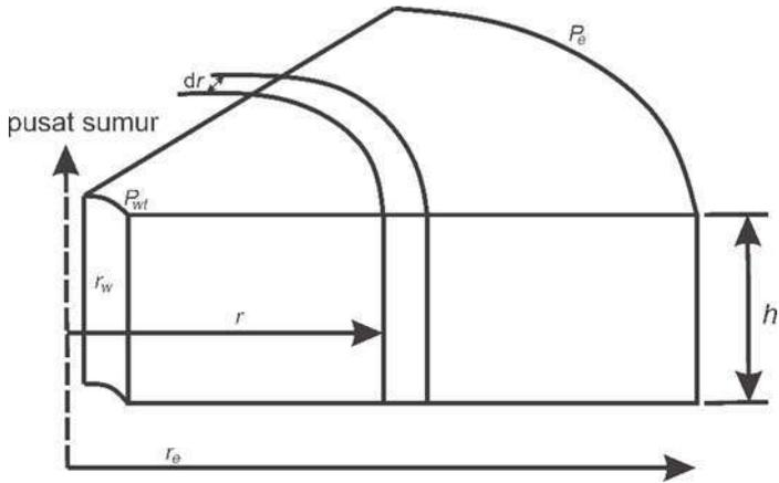
Gambar 6. 3 Aliran Radial
