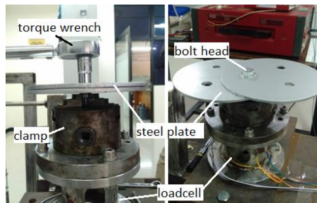
Figure 8. Set up for bolt torsion testing, position before wrench applied (right photo).
