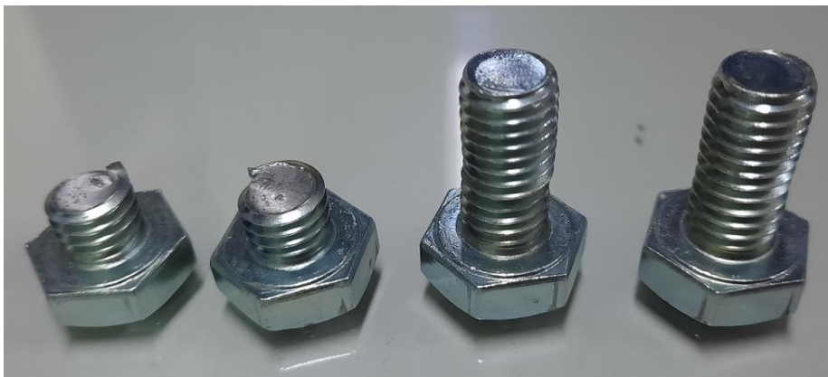
Figure 11. Bolt condition after testing, one at the right is condition before tested.
