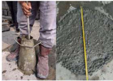
Fig.2 Workability testing of fresh concrete
