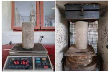
Fig.3 Dry density and compressive strength testing
