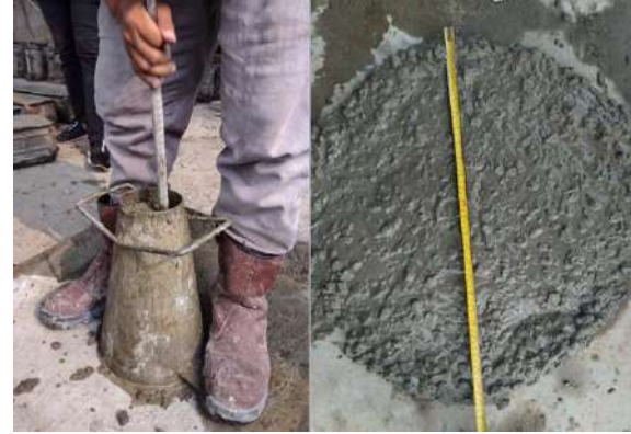
Fig.2 Workability testing of fresh concrete
