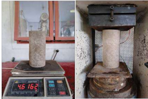
Fig.3 Dry density and compressive strength testing
