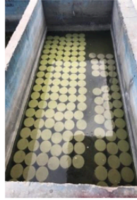
Fig. 3. Concrete samples on water curing.
