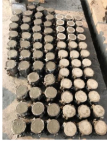
Fig. 2. Concrete samples on preparation.
