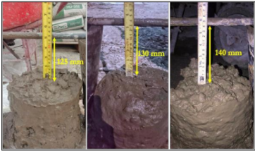
Fig. 2. The slump test results for each mixture
