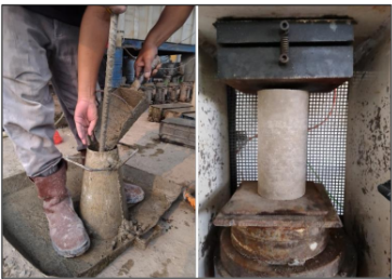
Fig. 1. (A) Slump Test (B) Compressive test
